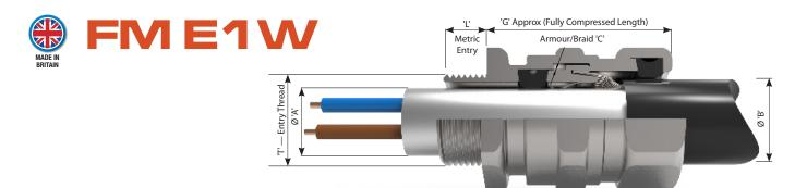
A fire resistant, robust and simple dual compression gland for applications using SWA or AWA cable in a heavy industrial, critical safety environment which is exposed to dust or extreme weather conditions. All cable glands can be supplied with a shroud, lock nut, serrated washer and an earth tag.
