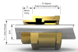
A robust and simple design for applications using non armoured cable in a heavy industrial environment which is exposed to dust or extreme weather conditions. All cable glands can be supplied with a shroud, lock nut, serrated washer and an earth tag.
